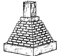
Belling out for bearing width.
