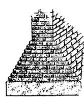
Belling out for bearing width.
