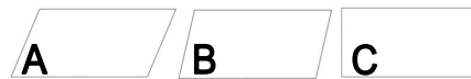
Figure 2: Angled tiles A (67°), B (71°), and C (90°) were hand cut using wooden templates
